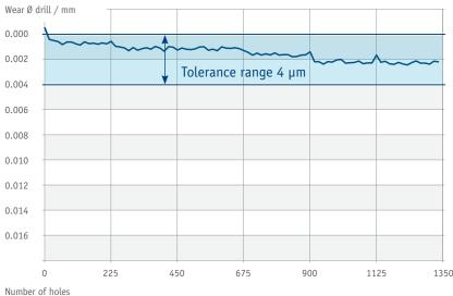
The trend towards miniaturization has reached mechanical components and requires increasingly smaller dimensions. The use of Ziroxit® ceramic milling tools allows the machining of precision components by means of CNC micro milling with long service life while continuously keeping to tight tolerances in the micron range.
